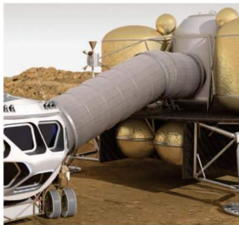
Fig. 13 Tunnel ingress method developed as a part of the National Aeronautics and Space Administration’s Evolvable Mars Campaign.
