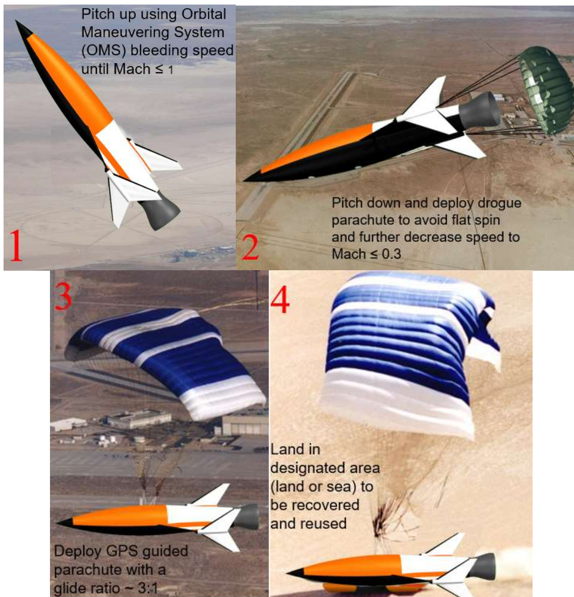
Figure 13.2.1: Baby Jay landing procedure
