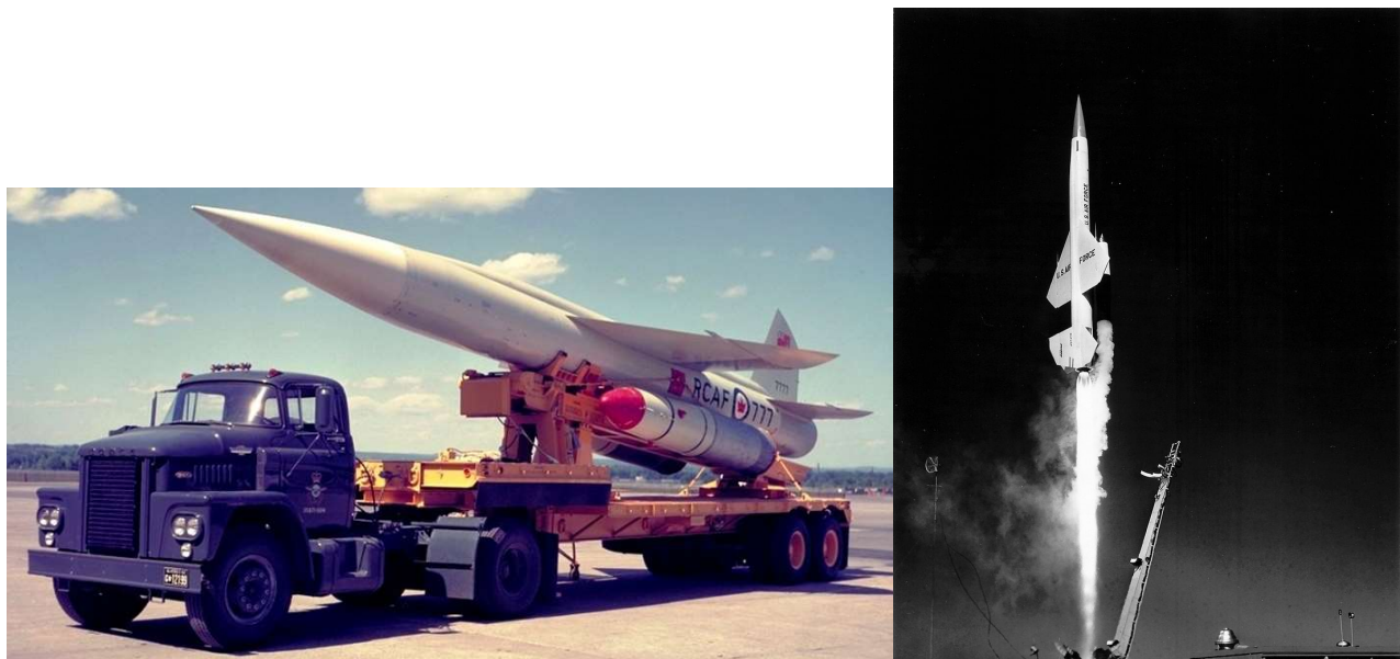
Figure 25.4: Bomarc missile transportation and launch systems [33,34]
