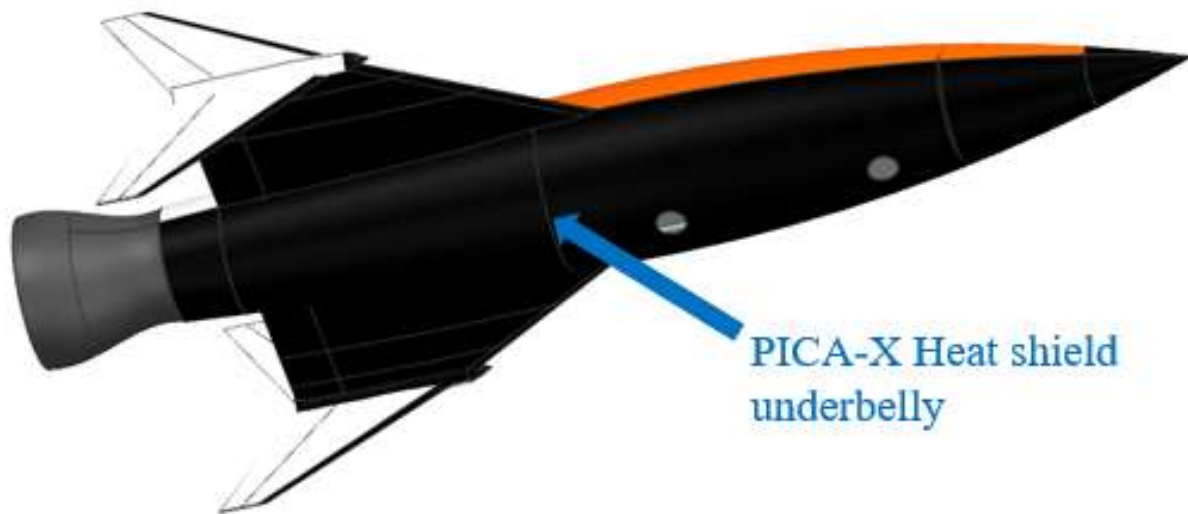
Figure 13.1.2: PICA-X heat shield on Baby Jay Underbelly
