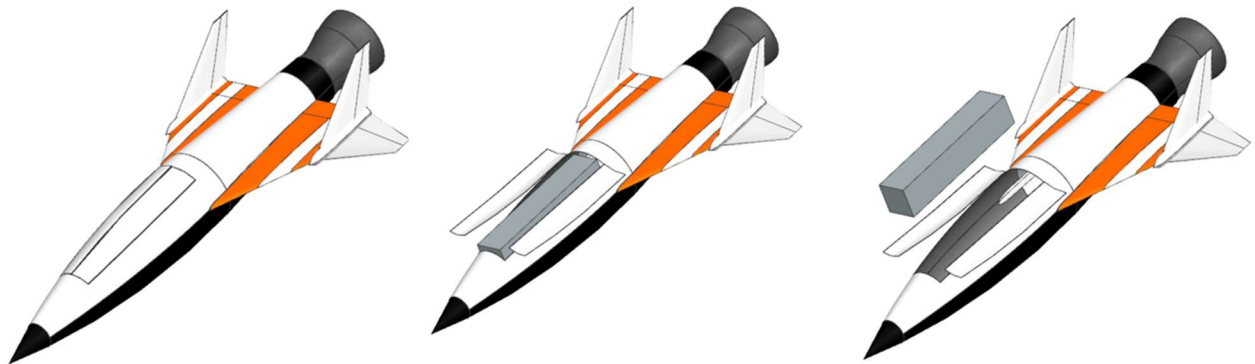
Figure 25.3: ISR payload removal or replacement
