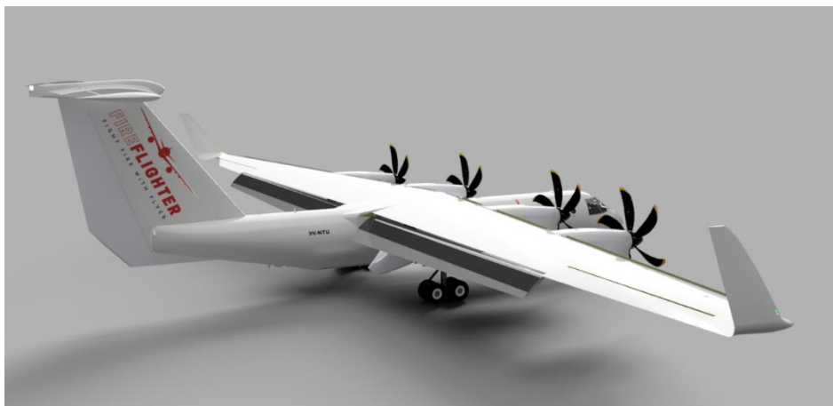
Figure 15: Rear view with flaps extended to 40 degrees (full extension).
