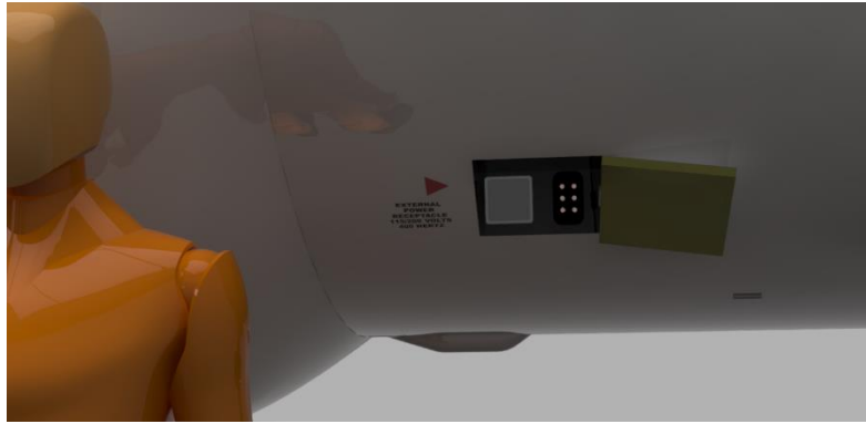
Figure 67: External power door open
