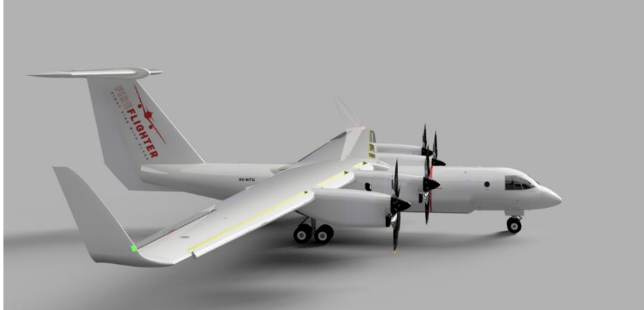
Figure 14: Slats extended to 30 degrees.
