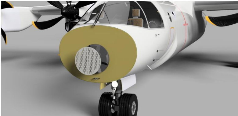
Figure 64: Weather and terrain radar in the nose of the aircraft
