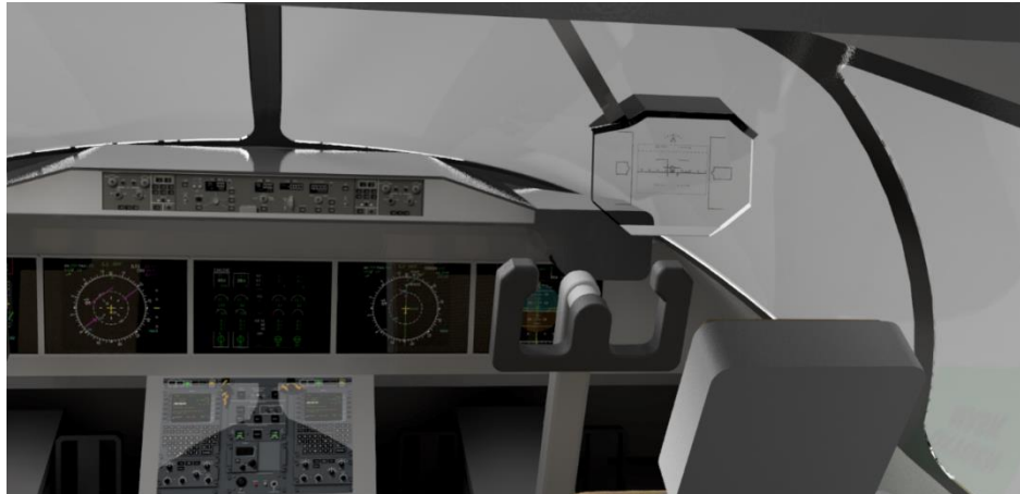
Figure 75: Glass cockpit and head-up display unit.
