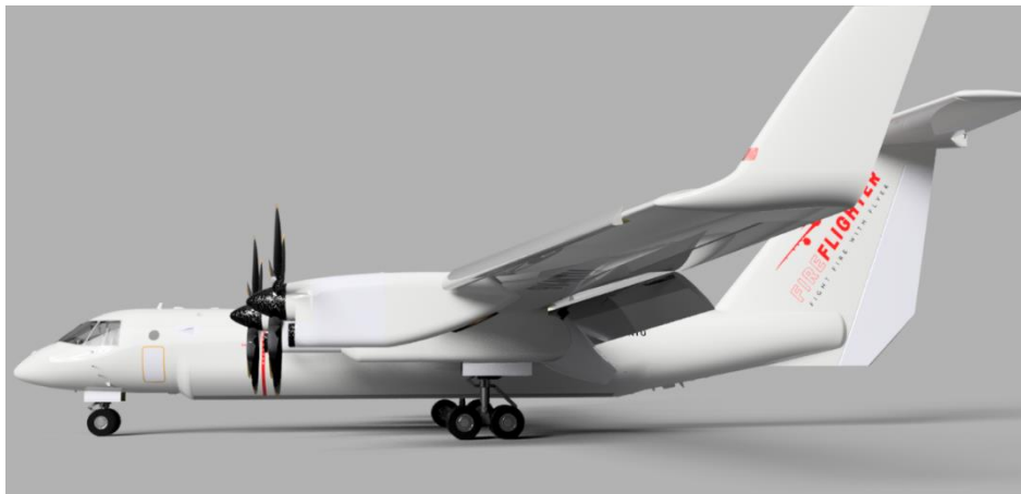
Figure 16: Side view of flaps extended to 40 degrees (full extension). Note inboard nacelle deflects together with flaps.
