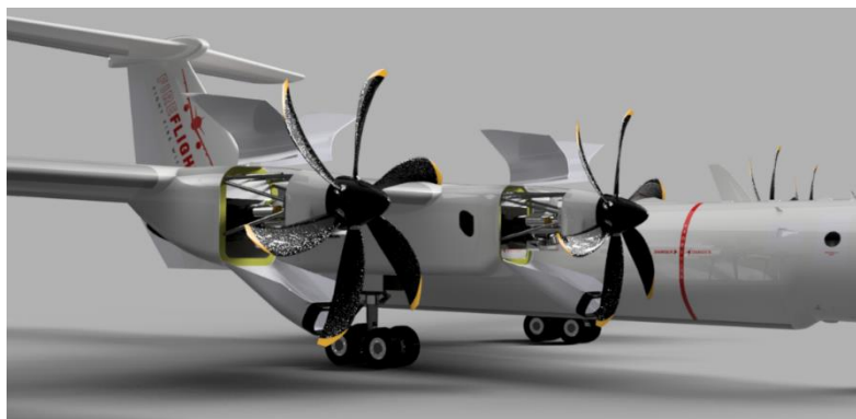
Figure 21: Open maintenance panels on both sides and lower part of the nacelle. Engine truss structure can also be seen.
