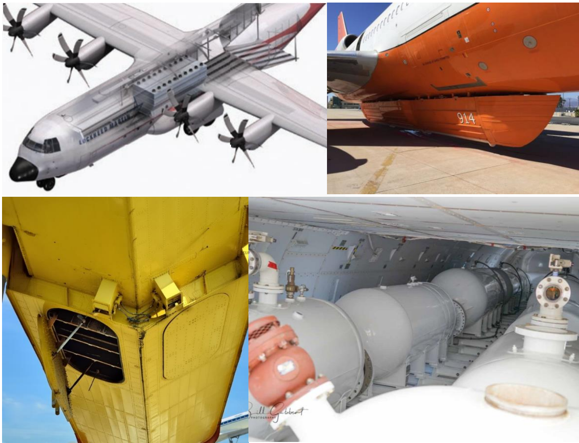
Figure 28: Types of retardant delivery systems. From top left, clockwise: Internal Discrete Tank in a C-130 [60], External Discrete Tank on a DC-10 [61], Integral Tank on a CL-415 [62], Internal Pressurised Tank in the 747 SuperTanker [63].
