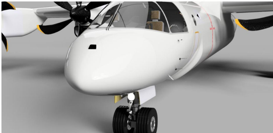
Figure 77: Enhanced Vision System located on the nose of the aircraft.
