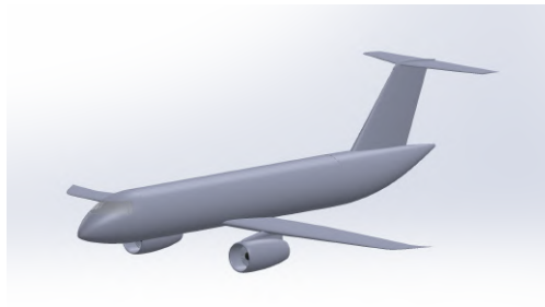
Fig. 13 Low-Wing Configuration with Engines Mounted to the Bottom of the Wing
