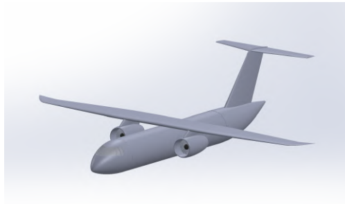
Fig. 14 High-Wing Configuration with Engines Mounted to the Bottom of the Wing
