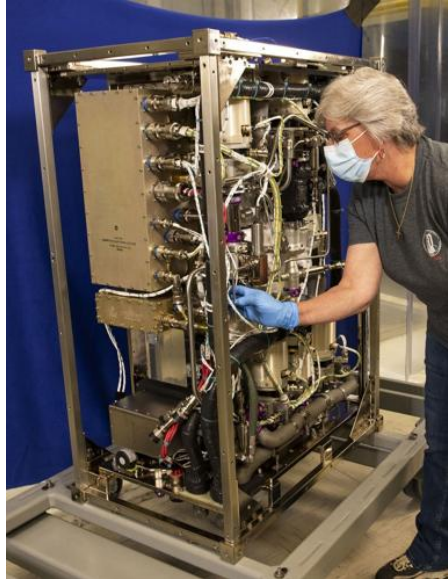
Figure 9: Four bed carbon dioxide removal unit [24]. This will be used to ensure the crew is not exposed to dangerous levels of carbon dioxide.
