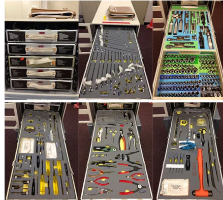
Figure 15: The ISS toolbox is shown here. It contains wrenches, a ratchet, sockets, drive accessories, screwdrivers, specialty sockets, pliers, cutters, tweezers, files, hammers, snips, a saw, and pry bars [55].
