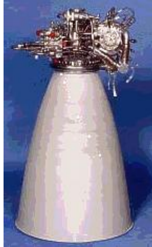
Figure 19: Colored picture of the XLR 132. The dimensions of the XLR 132 are near identical to that of the Transtar III, thus it is used as a representation of what the engine would likely be like in appearance. [63].
